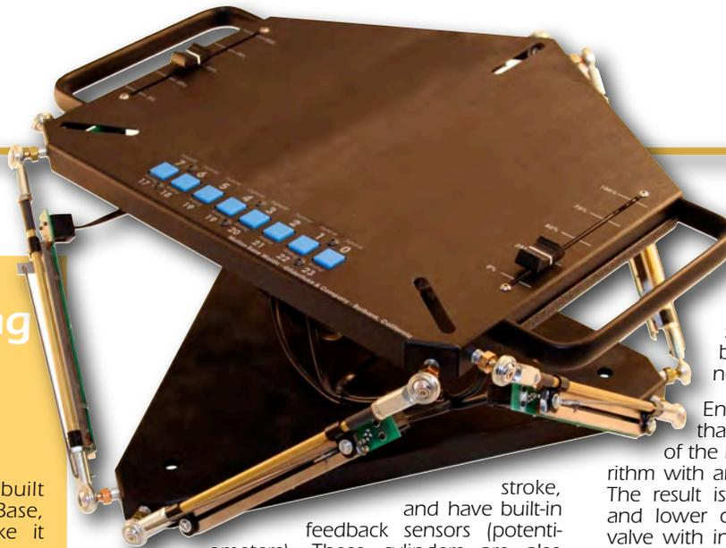
stroke, and have built-in feedback sensors (potentiometers). These cylinders are also available with non-contact types of position sensors, which will potentially last much longer. Moving from the 6" stroke cylinders to 12" stroke cylinders or to a slightly larger bore cylinder would result in a larger base, for only a small amount more cost for the longer cylinders.
