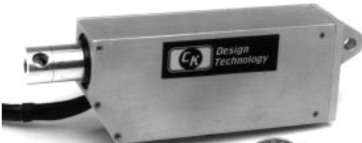
Typical of these new actuators are their new two inch stroke 'Mini' linear actuators. They are about 4-1/2" long, less than 1" thick, and 1-1/2" tall, and come in two load ratings: The first has a six pound operating load rating (20 pound stall) and moves at a speed of six inches per second. The second has a twelve pound operating load rating (35 pound stall) and moves at a speed of three inches per second.
