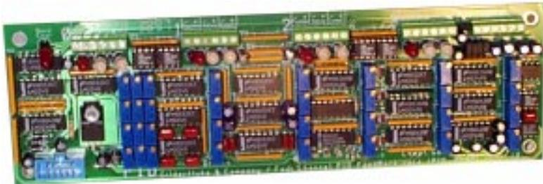
**New PID-Quad Electronic Feedback Card**
