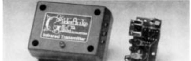
The infrared (IR) transmitters are placed along the vehicles' path, and continuously broadcast requests for specific messages to be played. As an IR receiver and Digital Audio Repeater-equipped vehicle pass each transmitter, it picks up the signal and plays the appropriate sound or message. Typical applications are on trains, dark rides, trams, monorails, rollercoasters, subways, and a variety of mass transit systems. Each repeater can hold up to 255 messages of virtually any length.
